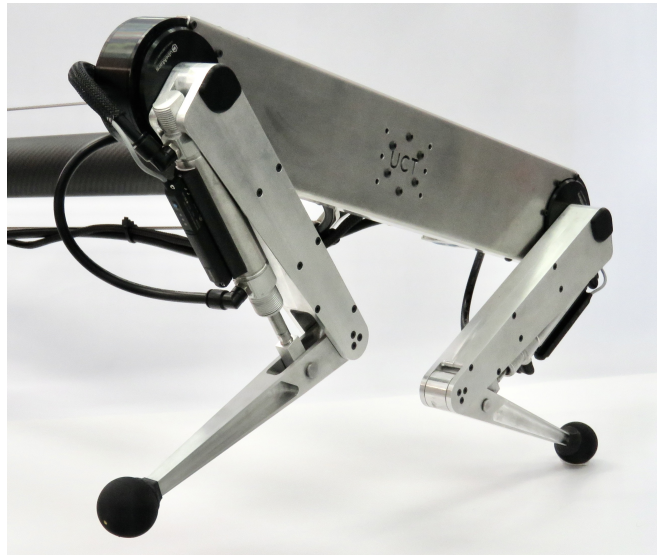
Fig. 1. Kemba , a hybrid electric and pneumatic legged robot designed for rapid maneuvers.
